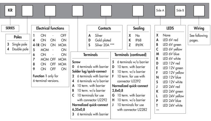
\*\*\* S contacts for all functions except 5 and 4-1R - for normalized quick-connect terminals 6,35x0,8 only.
