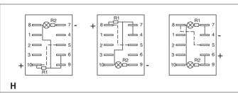
To obtain 2 symbol illumination levels (night illumination when OFF and higher illumination when ON).
