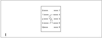
To have a polarity inversion (typical application : fan motor).
